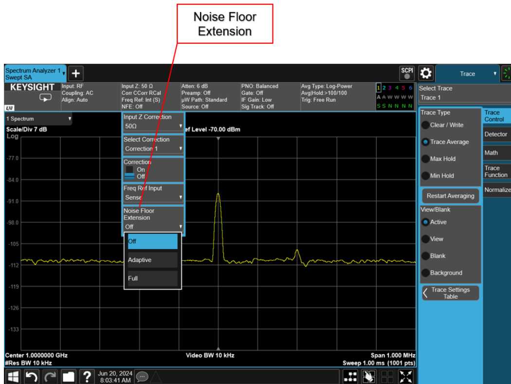
Figure 4. Next, press the “Noise Floor Extension” softkey and choose either “Adaptive” or “Full”. Additionally, turn on trace averaging with a sufficient number of trace averages ( \geq 10 averages)
