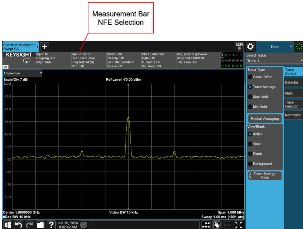
Figure 3. In this scenario a fundamental signal is detected at 1 GHz as well as two lower-level signals seen on either side. Increasing the SNR would make the lower-level signals more visible. A quick way to increase the SNR is to lower the noise floor. A quick way to lower the noise floor is to use NFE. Start by pressing the third measurement bar selection at the top.
